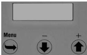
Switch on the mains switch and press the (-) key at the same time. Continue actuating the (-) key until the display is lightened.
