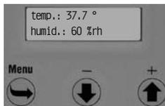
Switch on the mains switch and press the (+) key at the same time. Continue to actuate the (+) key until the display is lightened.
