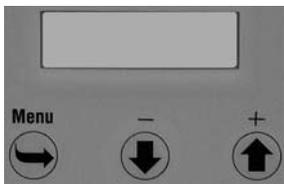
Switch on the mains switch and press the (menu) key at the same time. Continue to actuate the (menu) key until the display is lightened.
