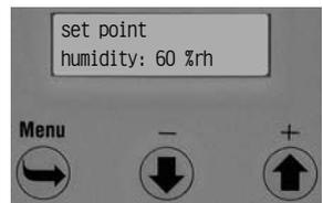
Set the required nominal value with the (+) or (-) key. A range of values from 30 to 90 % relative humidity is enabled. After the setting has been carried out the new values are immediately saved.
